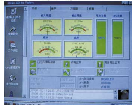
The type of information available from the 'Smart' UPSILON software for Windows and most other operating platforms.
